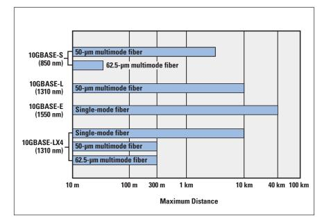
Figure 2: 10-Gbps Ethernet Distance Options (log scale)
