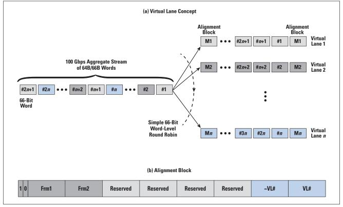
The virtual lanes are then transmitted over physical lanes. If the number of physical lanes is smaller then the number of virtual lanes, then bit-level multiplexing is used to transmit the virtual lane traffic. The number of virtual lanes must be an integer multiple (1 or more) of the number of physical lanes.
